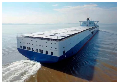
Fig. 2. Unmanned ship with horizontally mounted PV panels [13]
