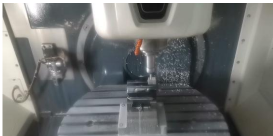
Fig. 4. Milling of test pieces
