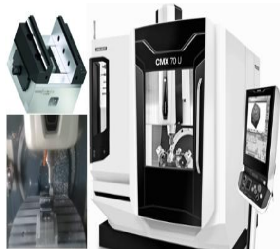
Fig. 1. CNC vertical machining center and vice used in experiments
