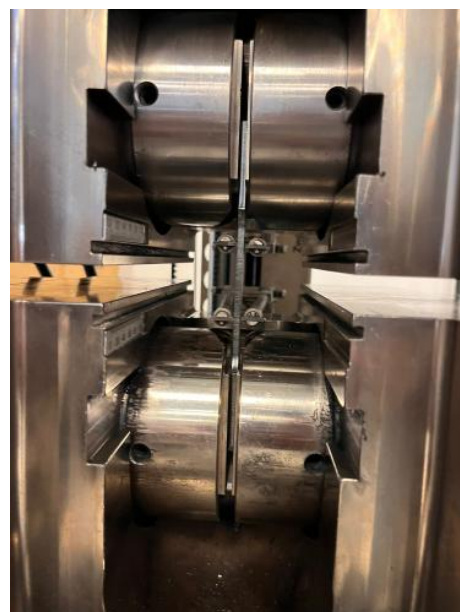
Fig. 1. Experimental tensile specimen used for calibration of the MISO model.
