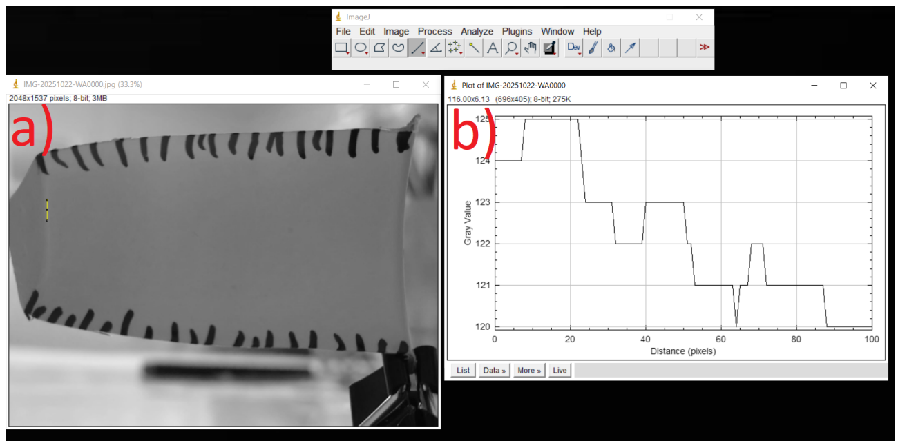
Fig. 4. (a) Selected ROI location on the thermoformed packaging sidewall, (b) the corresponding gray-scale intensity profile extracted using ImageJ.
